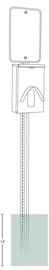
Using a post hole driver (not included), drive the sign post (C) approximately 15-18" into the ground. Make sure that the "hollow" or "recessed" side of the post is facing where you want the front of the unit to face. Use a level (not included) to ensure the pole is standing upright and will properly support the unit. Adjust if necessary.
